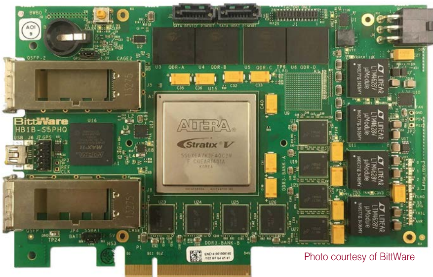
Altera Stratix V GX/GS Half-Length PCIe Board with Dual QSFP+/SFP+, DDR3 and QDRII+
