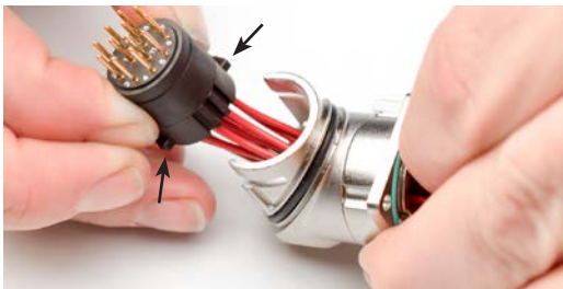
Step 5 - Locate keys on sides of insert
