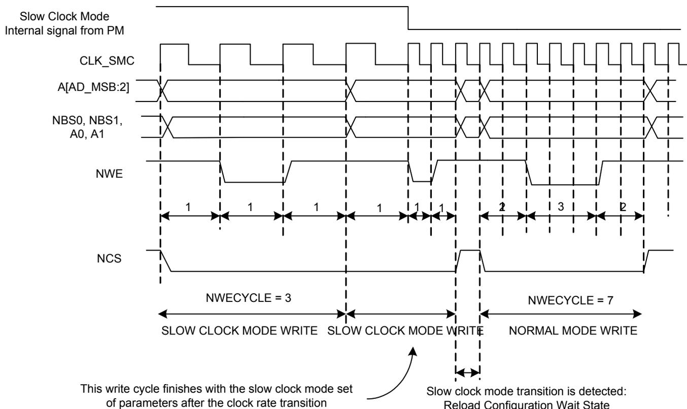
**Figure 18-32.** Recommended Procedure to Switch from Slow Clock Mode to Normal Mode or from Normal Mode to Slow Clock Mode
