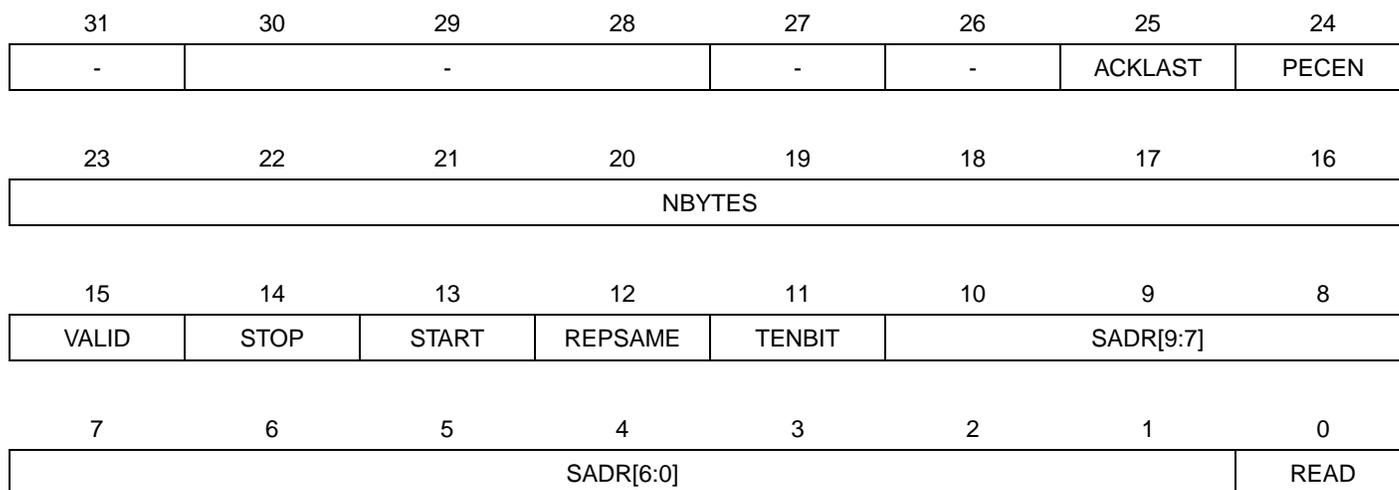
This register is identical to CMDR. When the VALID bit in CMDR becomes 0, the content of NCMDR is copied into CMDR, clearing the VALID bit in NCMDR. If the VALID bit in CMDR is cleared when NCMDR is written, the content is copied immediately.
