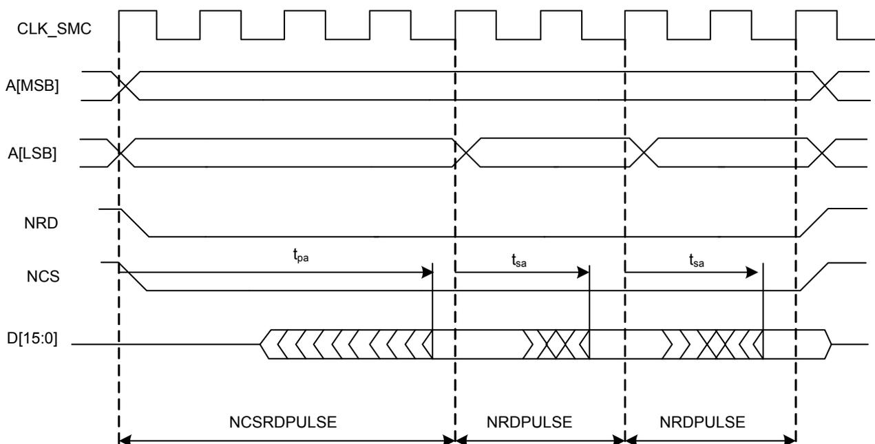
The NRD and NCS signals are held low during all read transfers, whatever the programmed values of the setup and hold timings in the User Interface may be. Moreover, the NRD and NCS timings are identical. The pulse length of the first access to the page is defined with the PULSE.NCSRDPULSE field value. The pulse length of subsequent accesses within the page are defined using the PULSE.NRDPULSE field value.
