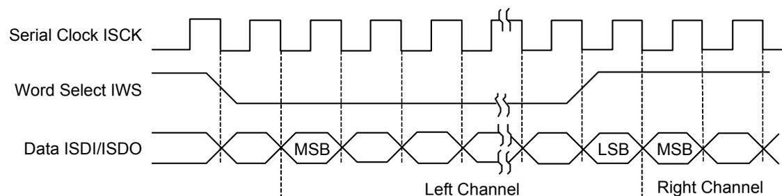
Data bits are sent on the falling edge of the Serial Clock and sampled on the rising edge of the Serial Clock. The Word Select line indicates the channel in transmission, a low level for the left channel and a high level for the right channel.
