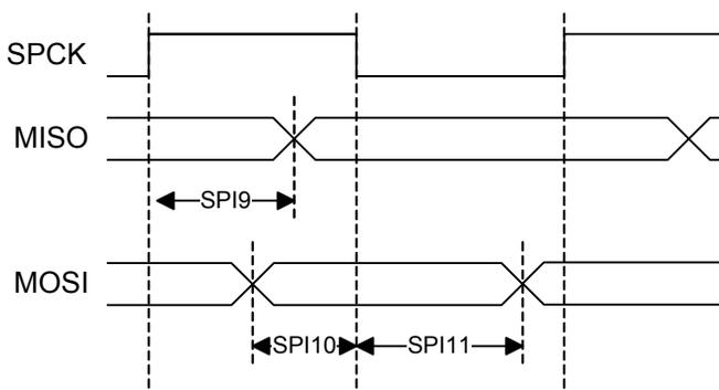
**Figure 40-15.** SPI Slave Mode NPCS Timing
