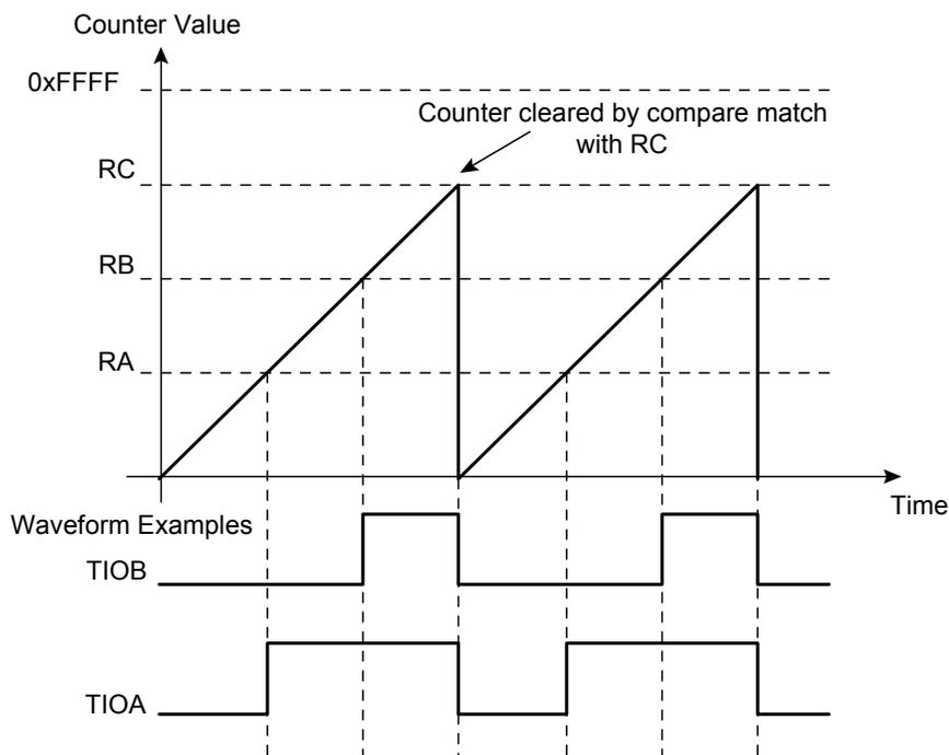
**Figure 31-9.** WAVSEL = 2 With Trigger
