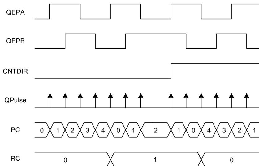
**Figure 34-6.** PC reset by QEPI signal (TOP.PCTOP = 79, CF.IDXPHS = "00", CF.IDXE = "1")
