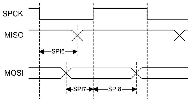
**Figure 40-14.** SPI Slave Mode With (CPOL= NCPHA= 0) or (CPOL= NCPHA= 1)
