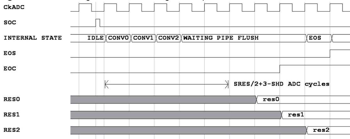
**Figure 36-5.** Using FRM and Converting at Full Speed
