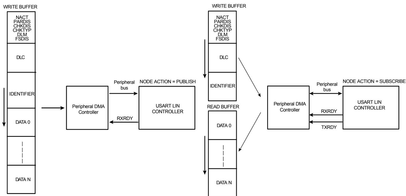
**Figure 25-52.** Master Node with Peripheral DMA Controller (PDCM=0)
