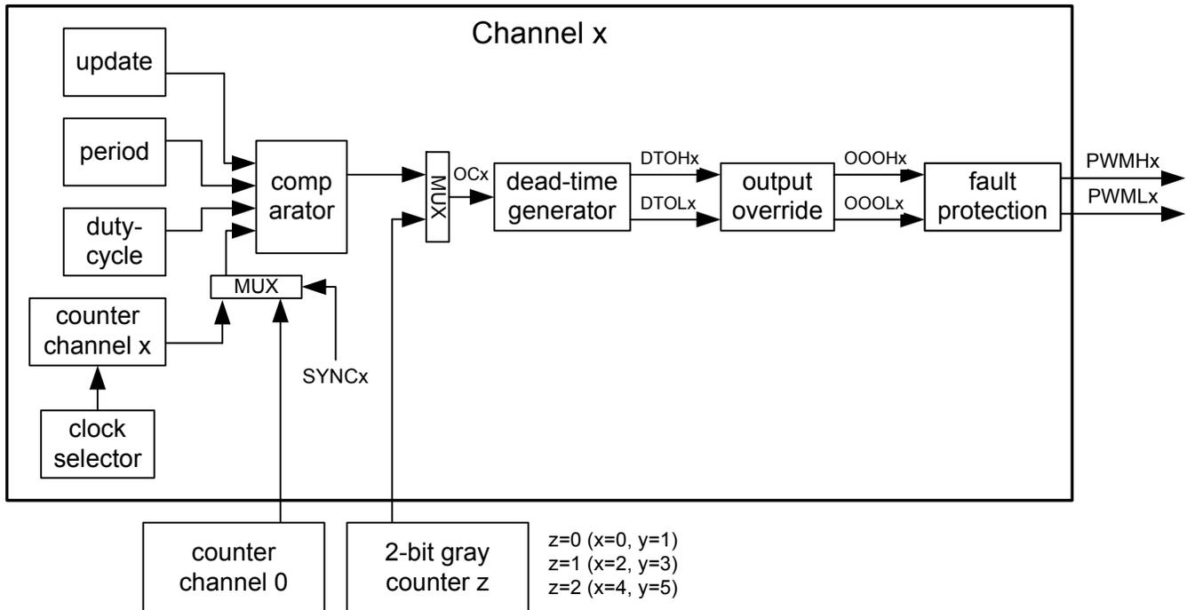
Each of the 4 channels is composed of six blocks:
