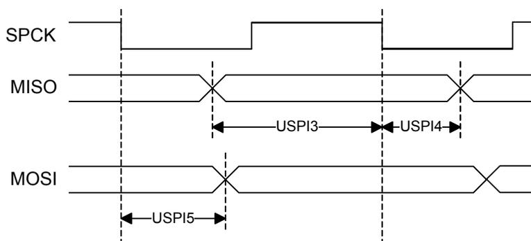
**Table 40-46.** USART in SPI Mode Timing, Master Mode<sup>(1)</sup>
