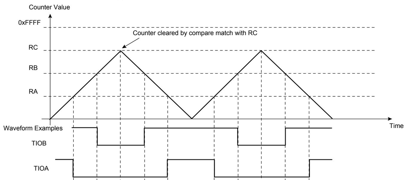
Figure 31-13. WAVSEL = 3 With Trigger
