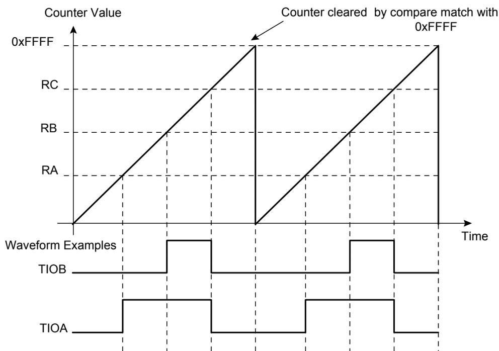
**Figure 31-7.** WAVSEL= 0 With Trigger
