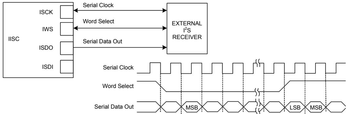
Figure 30-7. Codec Application Block Diagram
