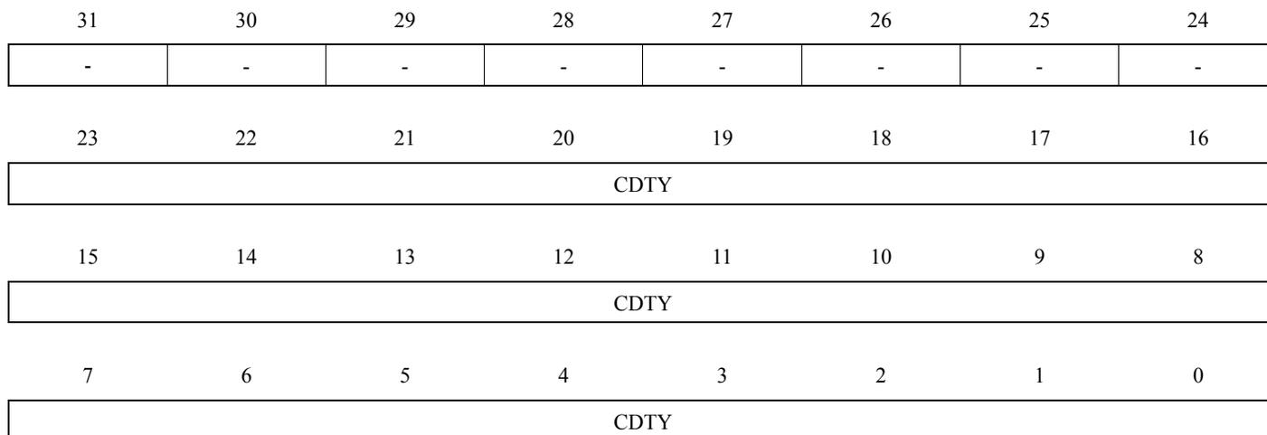
Only the first 20 bits (channel counter size) are significant.
