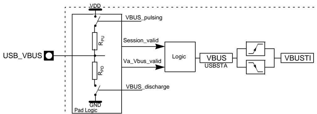
The control logic of the USB\_VBUS pad outputs two signals:
