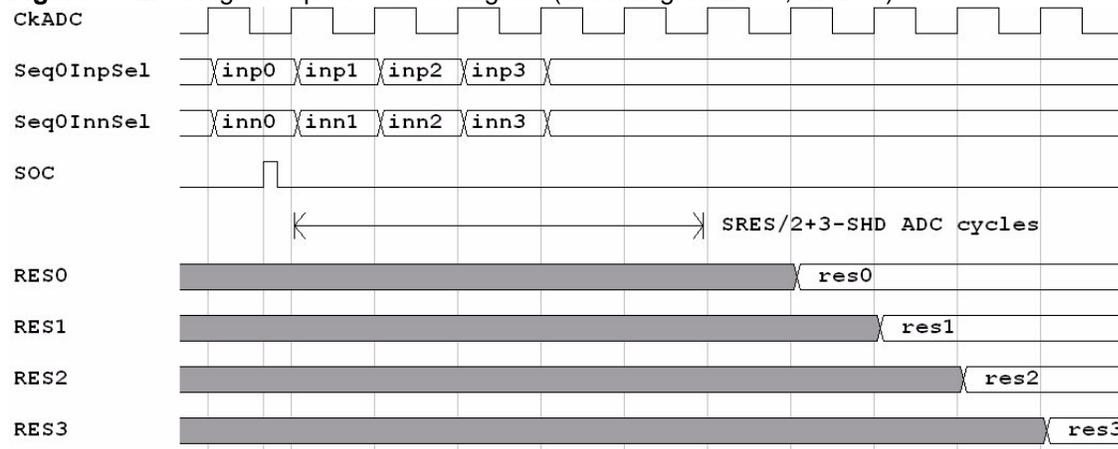
36.6.4.3 Dual-sequencer mode (simultaneous sampling)
