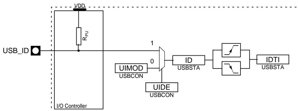
The USBC mode (device or host) can be detected by the USB\_ID pin or selected by writing to USBCON.UIMOD. This allows the USB\_ID pin to be used as a general purpose I/O pin even when the USBC interface is enabled.
