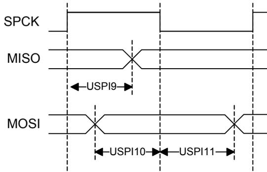
**Figure 40-10.** USART in SPI Slave Mode NPCS Timing
