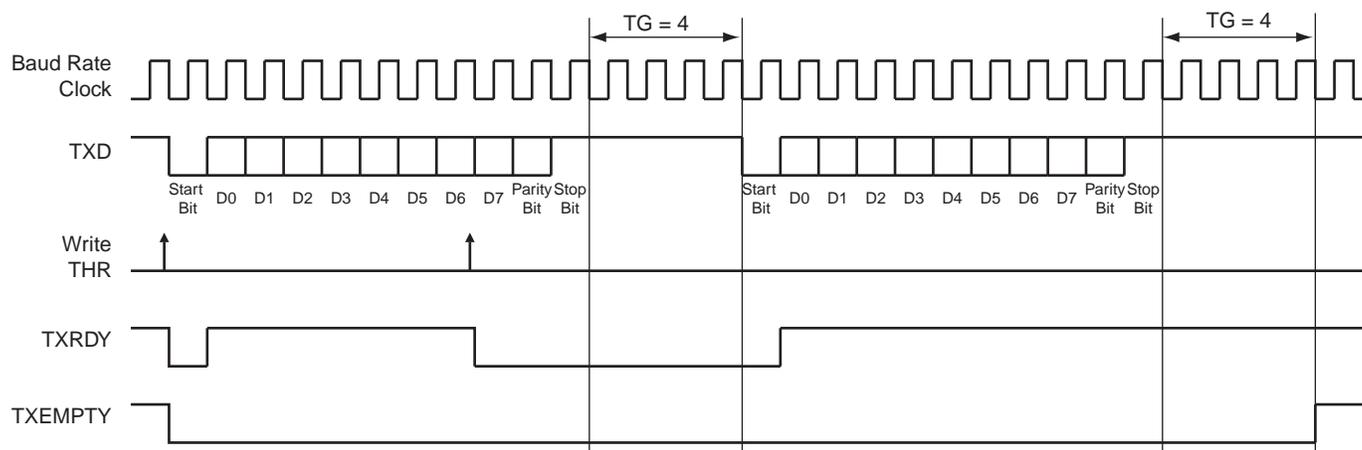
Table 25-8 indicates the maximum length of a timeguard period that the transmitter can handle in relation to the function of the Baud Rate.
