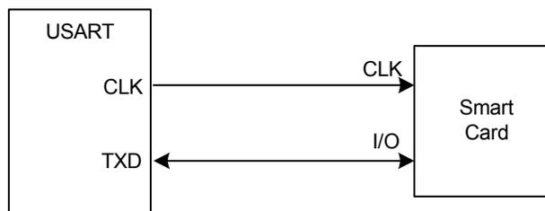
When operating in ISO7816, either in T = 0 or T = 1 modes, the character format is fixed. The configuration is 8 data bits, even parity and 1 or 2 stop bits, regardless of the values programmed in the CHRL, MODE9, PAR and CHMODE fields. MSBF can be used to transmit LSB or MSB first. Parity Bit (PAR) can be used to transmit in normal or inverse mode. Refer to ["Mode Register" on page 628](#) and ["PAR: Parity Type" on page 630](#).
