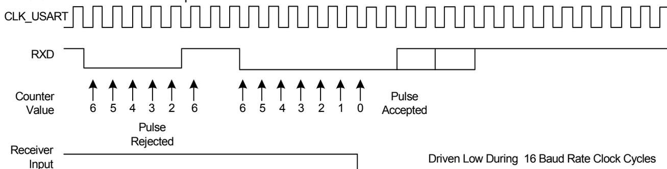
As the IrDA mode uses the same logic as the ISO7816, note that the FI\_DI\_RATIO field in FIDI must be set to a value higher than 0 in order to assure IrDA communications operate correctly.
