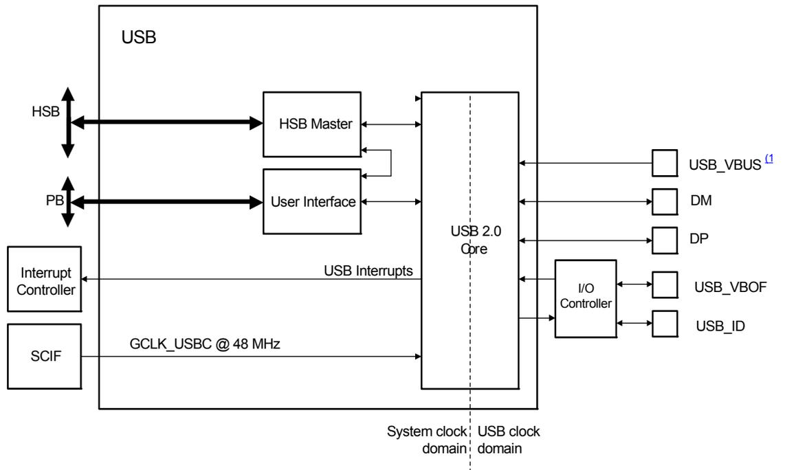
Note: The USB\_VBUS pin is 5V tolerant
