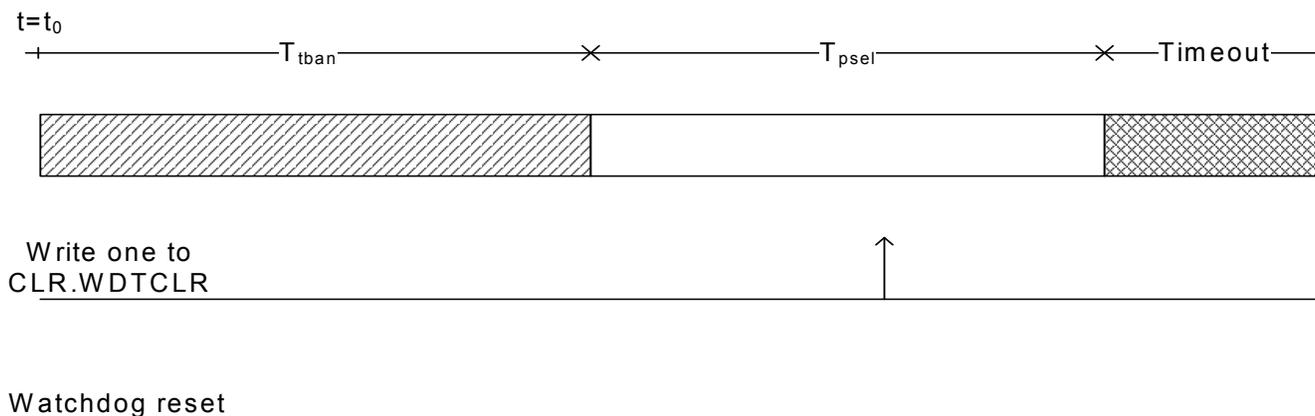
**Figure 10-5.** Window Mode WDT Timing Diagram, clearing within  $T_{\text{tban}}$ , resulting in watchdog reset.
