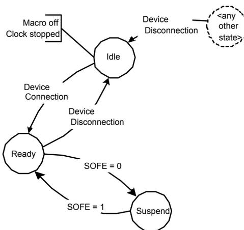
After a hardware reset, the USB host mode is in the Reset state (see [Section 32.6.1.1](#)).
