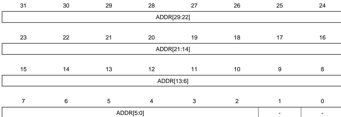
This register points to the entry in the receive buffer queue (descriptor list) currently being used. It is written with the start location of the receive buffer descriptor list. The lower order bits increment as buffers are used up and wrap to their original values after either 1024 buffers or when the wrap bit of the entry is set.
