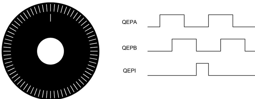
The phase signals are labelled QEPA and QEPB. If QEPA leads QEPB, the rotation direction is defined as positive. If QEPB leads QEPA, the rotation direction is defined as negative. Each time a line passes the sensor, a counter register (CNT.PC) is incremented or decremented depending of the rotation direction. A third input signal, QEPI, can be used to reset CNT.PC.
