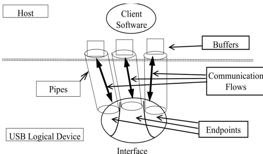
In host mode, the USBC associates a pipe to a device endpoint, according to the device configuration descriptors.
