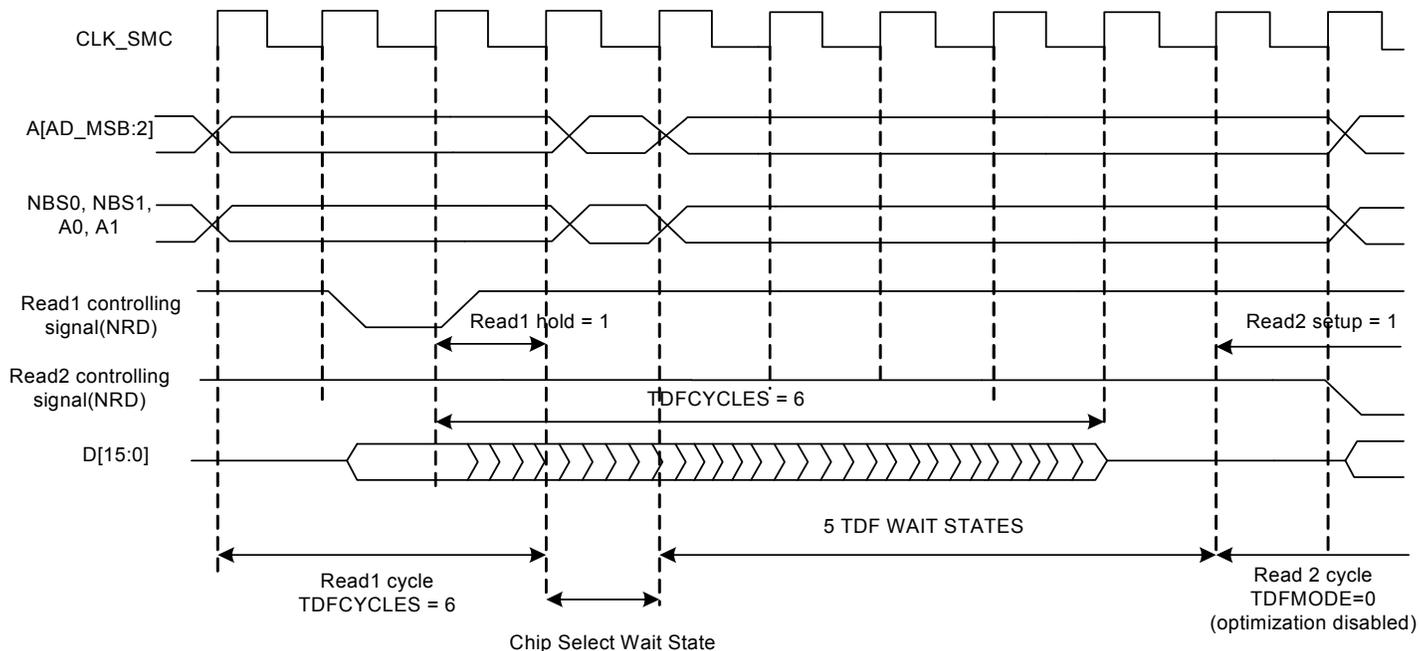
**Figure 18-23.** TDF Optimization Disabled (MODE.TDFMODE= 0). TDF Wait States between a Read and a Write Access on Different Chip Selects.
