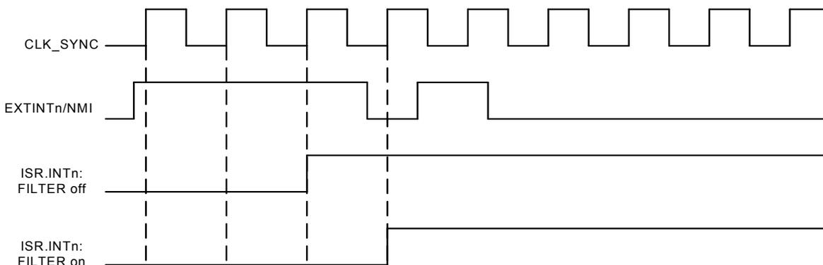
**Figure 12-3.** Timing Diagram, Synchronous Interrupts, Low Level or Falling Edge
