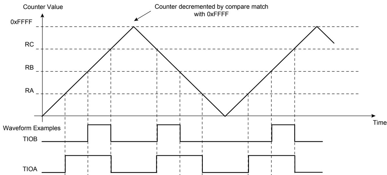
**Figure 31-11. WAVSEL = 1 With Trigger**
