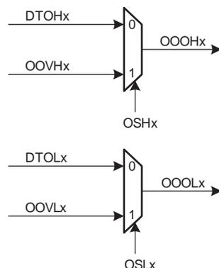
The OSHx and OSLx fields in the "Output Selection Register" on page 1016 (OS) allow the outputs of the dead-time generator DTOHx and DTOLx to be overridden by the value defined in the OOVHx and OOVLx fields in the "Output Override Value Register" on page 1015 (OOV).
