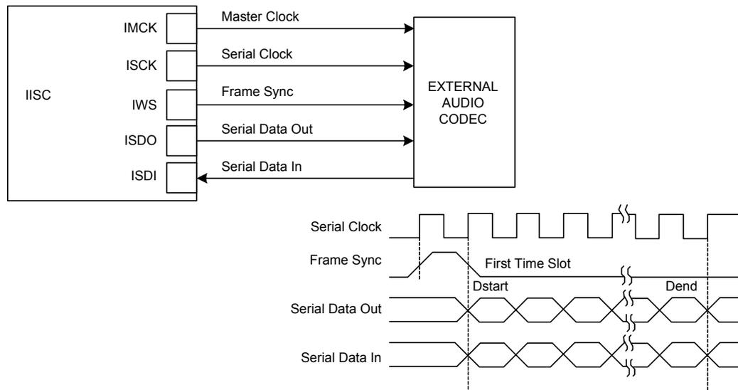
Figure 30-8. Time Slot Application Block Diagram
