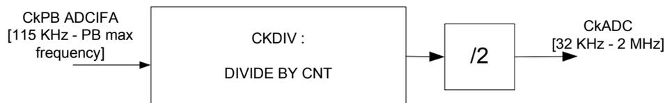
In addition when CKDIV is written, the internal counter is reset to avoid rollover phenomena: **DO NOT WRITE CKDIV WHEN PERFORMING CONVERSIONS.**
