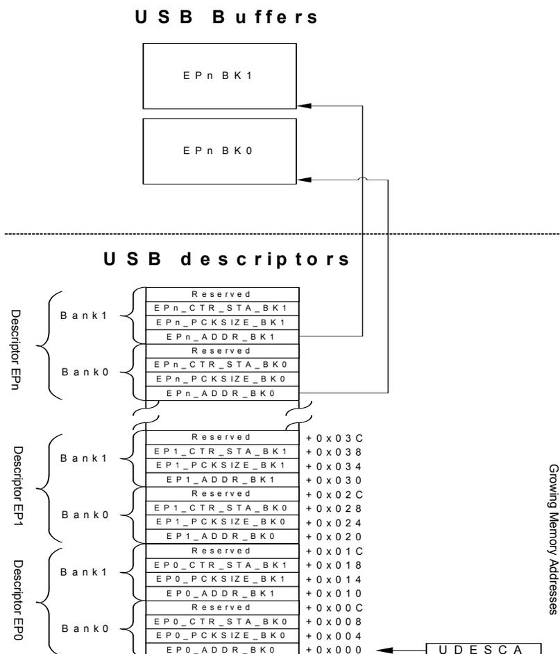
Each descriptor of an endpoint n consists of four words.
