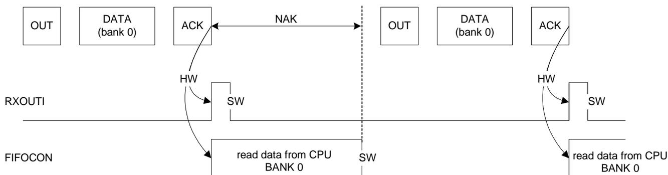
**Figure 32-15.** Example of an OUT endpoint with two data banks
