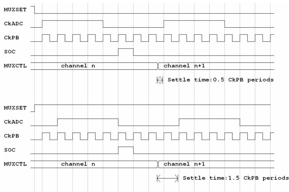
The chronogram above shows that for the same start of conversion (SOC) event, CkADC rises one PB clock period later. The ADC and S/H are sampling when CkADC is high, so setting the CFG.MUXSET bit will delay the sampling phase by one PB clock period.
