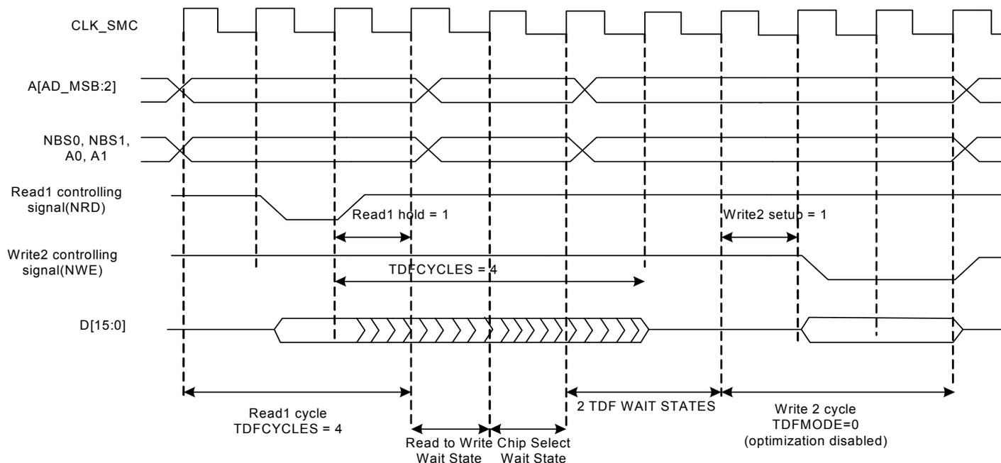
**Figure 18-24.** TDF Optimization Disabled (MODE.TDFMODE = 0). TDF Wait States between Read and Write accesses on the Same Chip Select.
